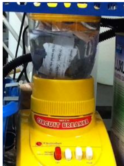
Figure 3.9: Water enters the blender to soak paper for 30 s
