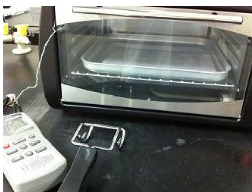
Figure 3.2: Temperature in oven is observed using thermocouple
