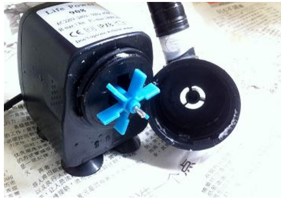
Figure 3.15: Magnetic drive pump mechanism
