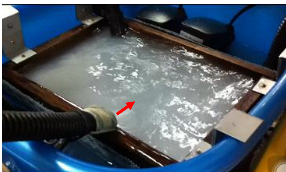
Figure 3.12: Water circulation by pump to make layer of pulp sheet even
