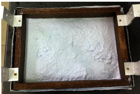
Figure 3.19: Pulp sheet is in contact with wet pulp moulding frame
