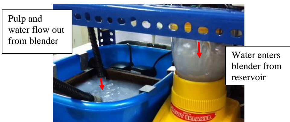
Figure 3.11: Pulp in the blender is transferred to pulp moulding frame while water is continuously flow from reservoir via blender to pulp moulding frame
