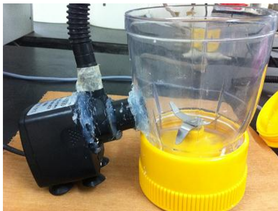
Figure 3.14: Magnetic drive pump is fitted to the blender jar
