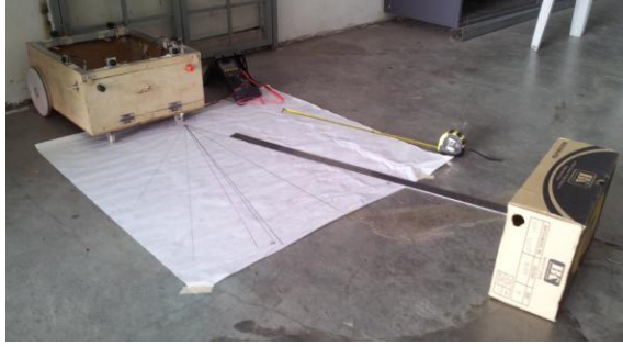
Figure 4.10: Sensor Coverage Test Setting
