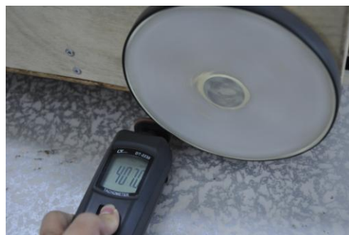
Figure 4.32: Determined rpm with Contact Tachometer
