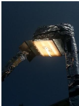
**Figure 3.24: Commercialized solar cell mounted to the cooling block**
