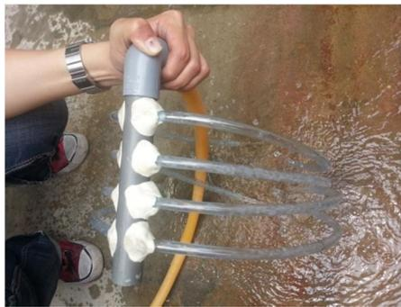
**Figure 4.21: Leaking test performed for the manifold**
