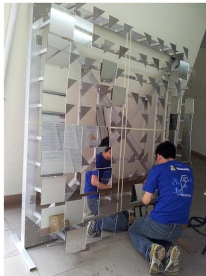
**Figure 4.25: Completed main frame with mirror being set on it.**
