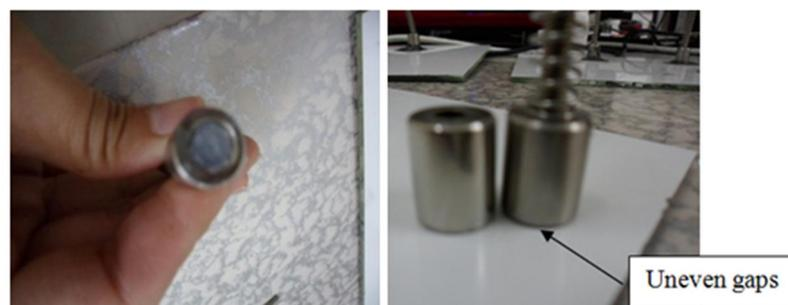
**Figure 3.14: fully filled silicon with bad finishing causes uneven surface**
