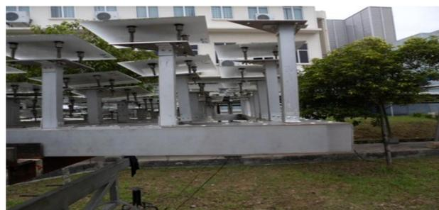
**Figure 4.23: Square aluminium bar with L bar fixed on it and also triangular plate for mirror tilting purpose**
