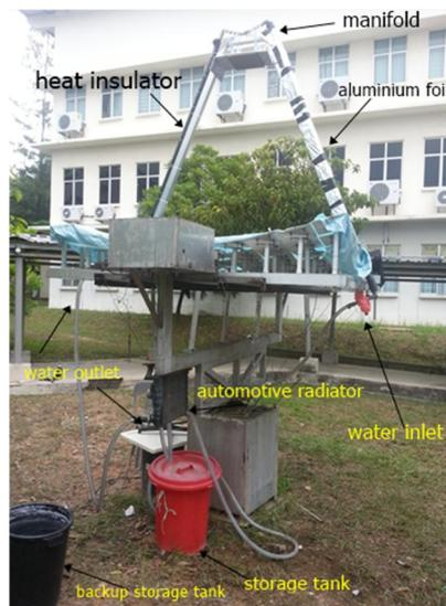
**Figure 4.20: Side view of CPV system with the whole cooling system**
