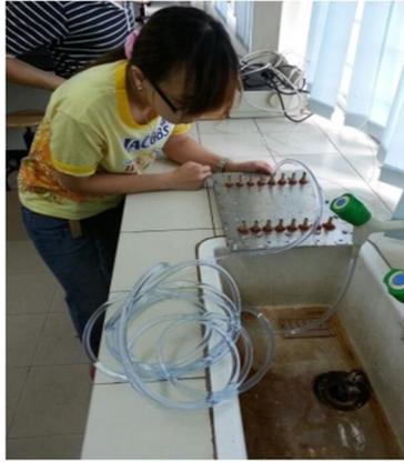
**Figure 4.19: Leaking test performed for the cooling block.**
