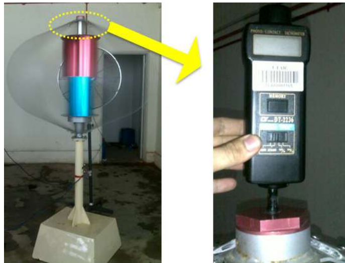
Figure 3.21: Measuring the rotor's speed of VAWT through Tachometer
