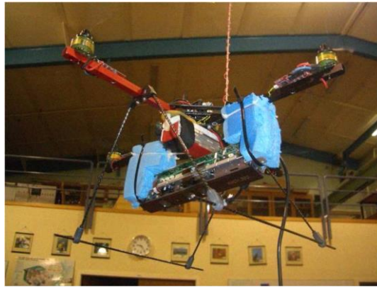
Figure 2-13: Kinect Sensor on Quadrotor Helicopter
