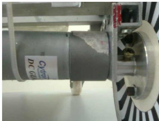
Figure 4-27: DC Motor and Shaft-Wheel Coupling
