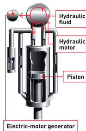
Figure 2.7: Inside of a GenShock shock absorber
