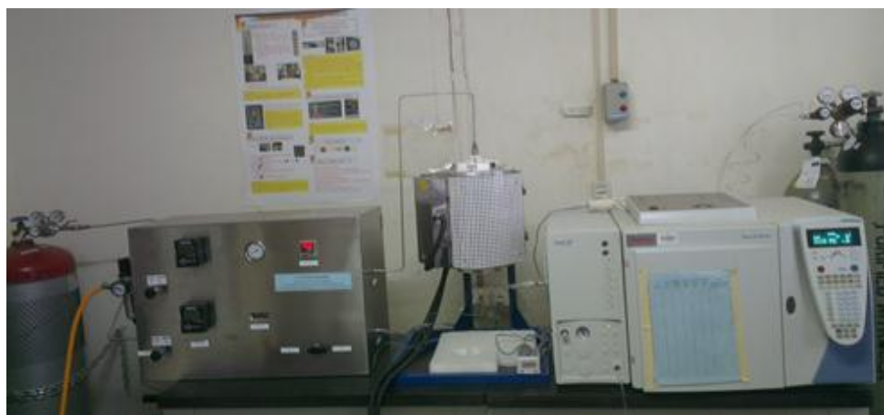
Figure 3.14: Fixed bed reactor coupled with Trace GC Ultra
