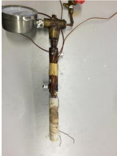
(a) Water cooled thermosyphon (HP1)
