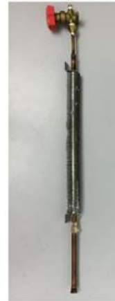
(b) Air cooled thermosyphon (HP 2&3)
