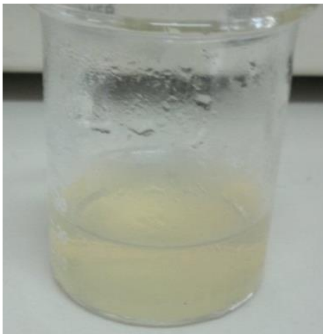
Figure 4.1: Synthesized silver nanoparticles in colloidal solution formulated with low concentration of stock material
