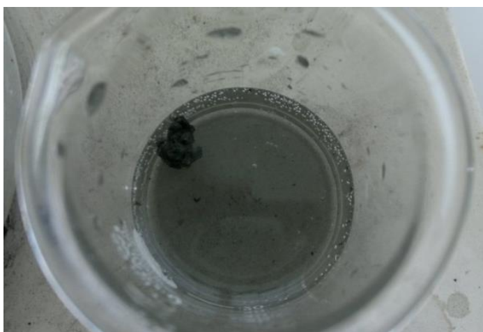
Figure 4.2: Agglomerated synthesized silver nanoparticles formulated with high concentration of stock material
