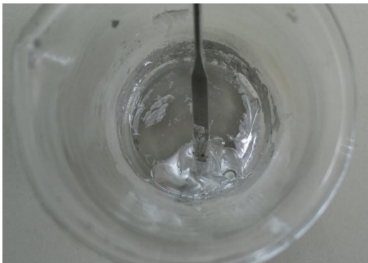
Figure 6.2: ICAs formulated with DGEBA resin and 0.8 weight fraction of filler contents
