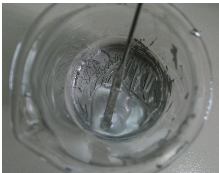
Figure 6.3: ICAs formulated with DGEBA resin and 0.6 weight fraction of filler contents
