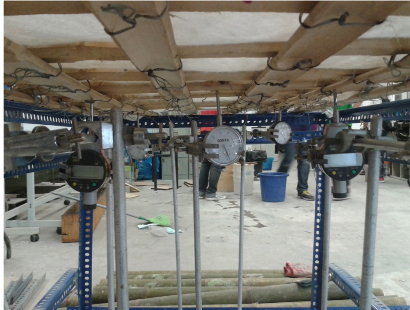
Figure 3.5: Set-up of dial gauges using retort stands and clamps
