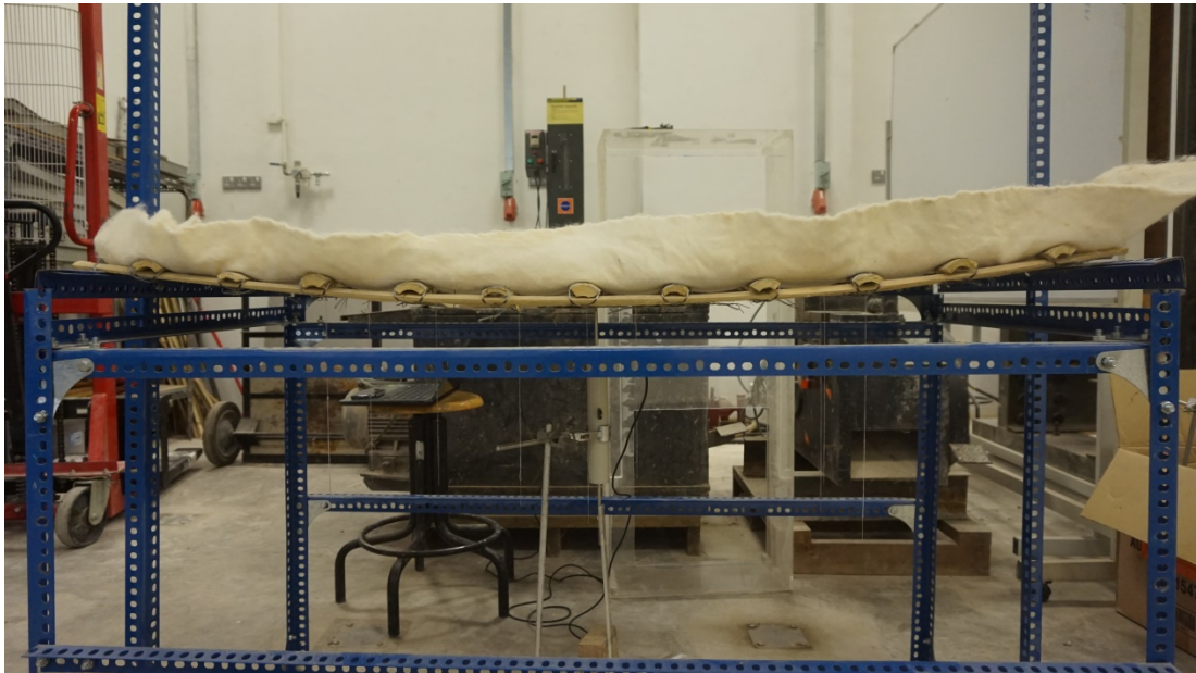
Figure C5: Deflection when sand load = 20 kg
