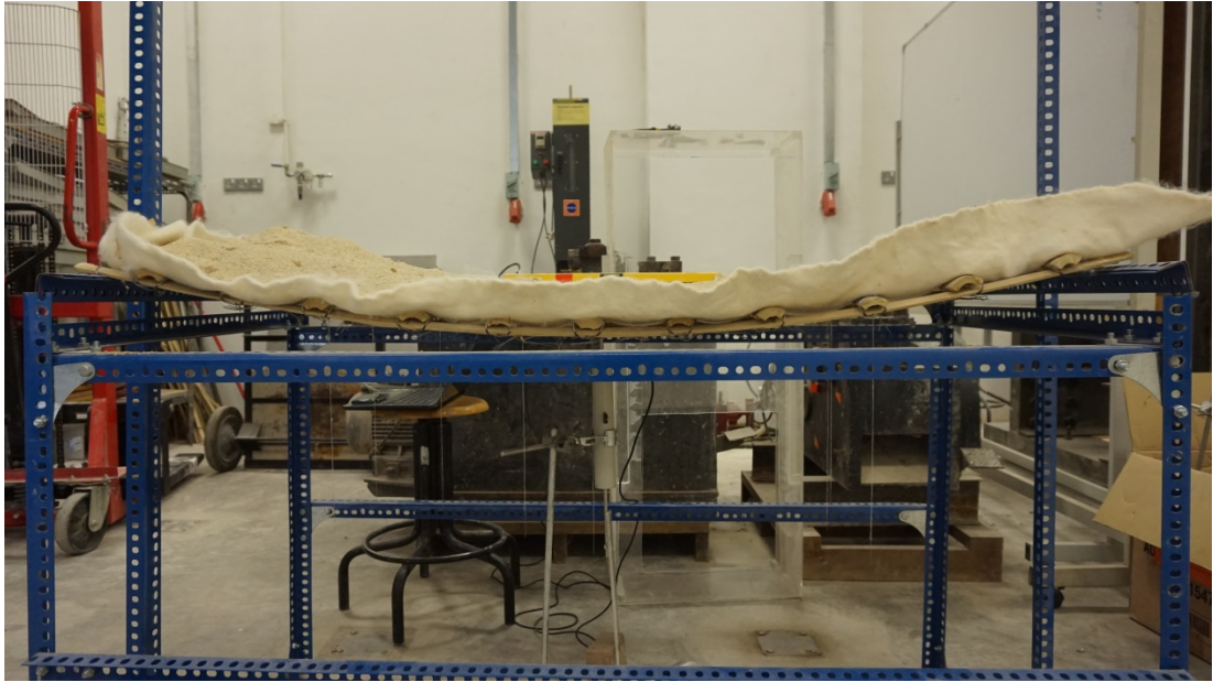
Figure C9: Deflection when sand load = 40 kg
