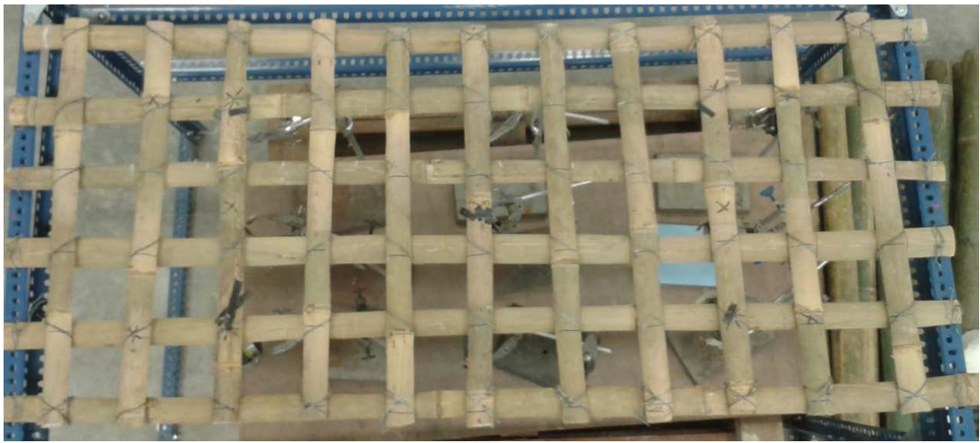
Figure 3.2: Bamboo grid simply supported on steel frame
