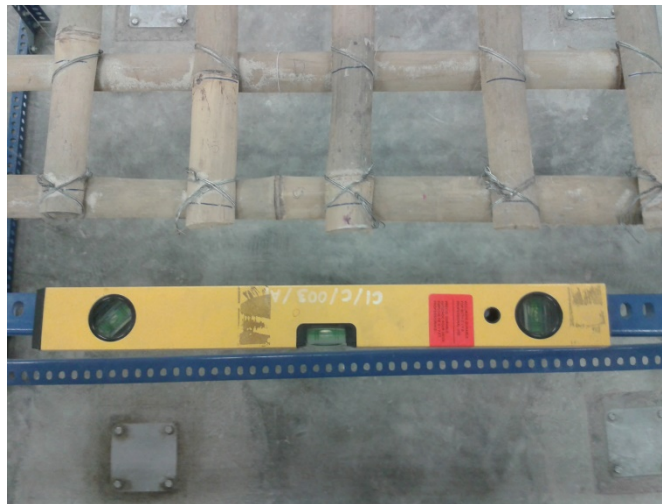
Figure 3.1: Magnetic level indicator
