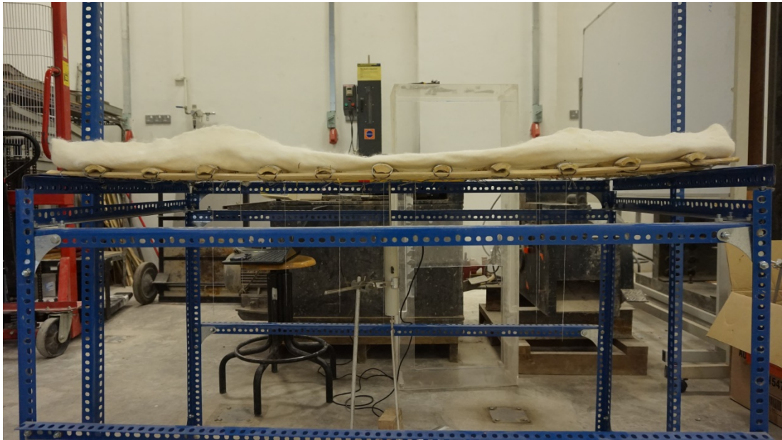
Figure C1: Deflection when sand load = 0 kg
