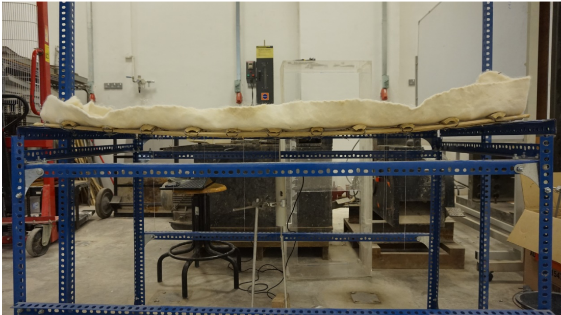
Figure C3: Deflection when sand load = 10 kg
