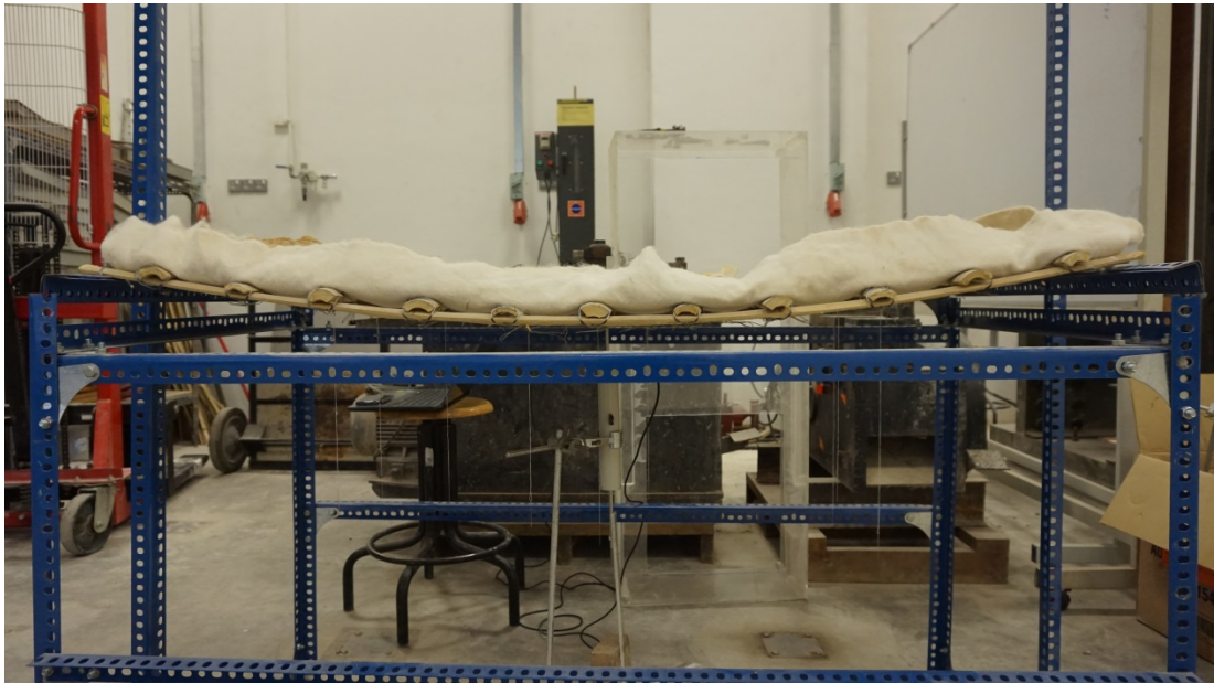
Figure C7: Deflection when sand load = 30 kg
