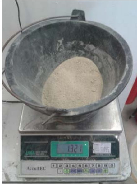
Figure 3.9: Weighing of dry sand using a weighing machine
