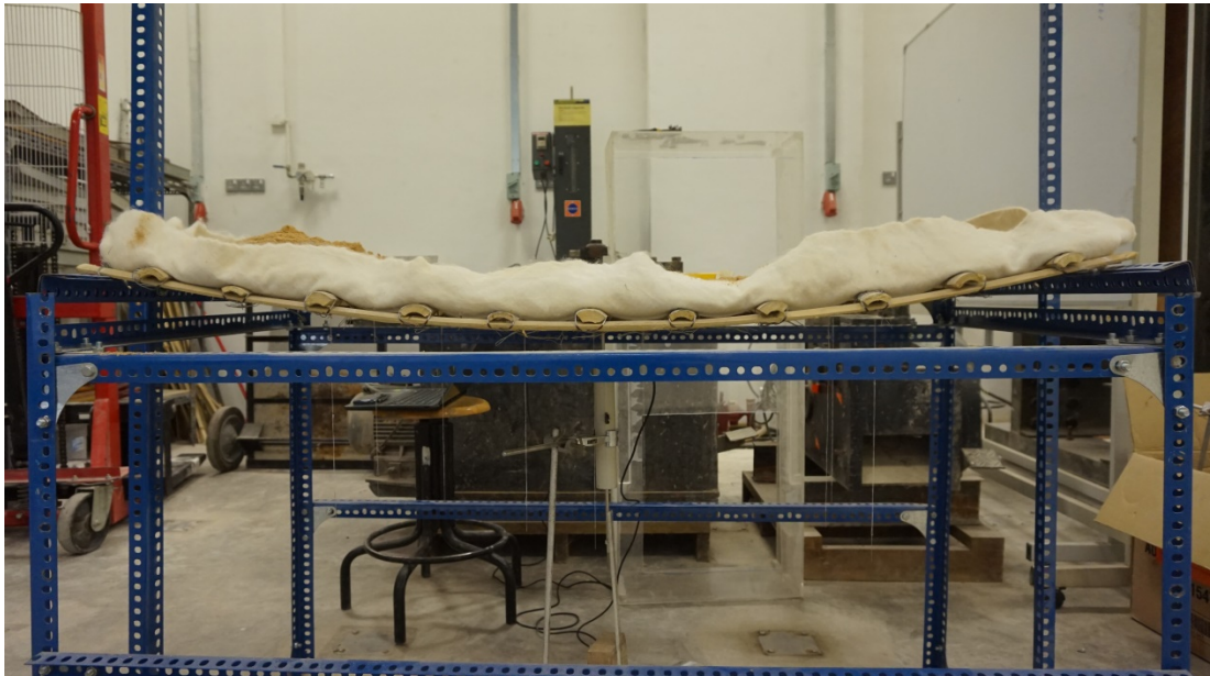
Figure C8: Deflection when sand load = 35 kg
