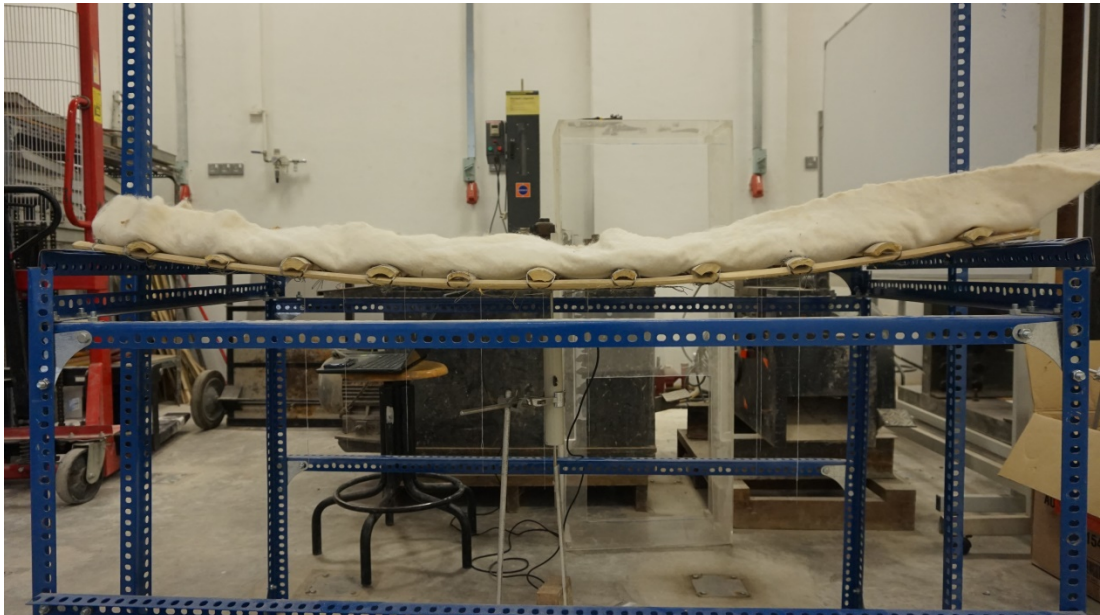
Figure C6: Deflection when sand load = 25 kg
