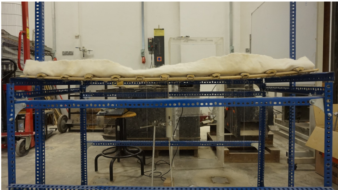
Figure C2: Deflection when sand load = 5 kg
