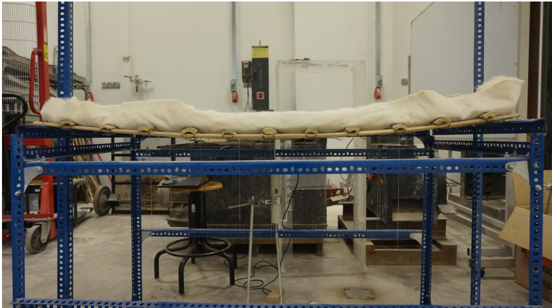
Figure C4: Deflection when sand load = 15 kg
