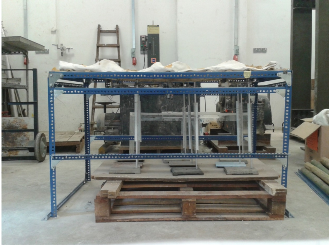
Figure 3.18: Steel frame before modification (loaded up to 20 kg of sand)
