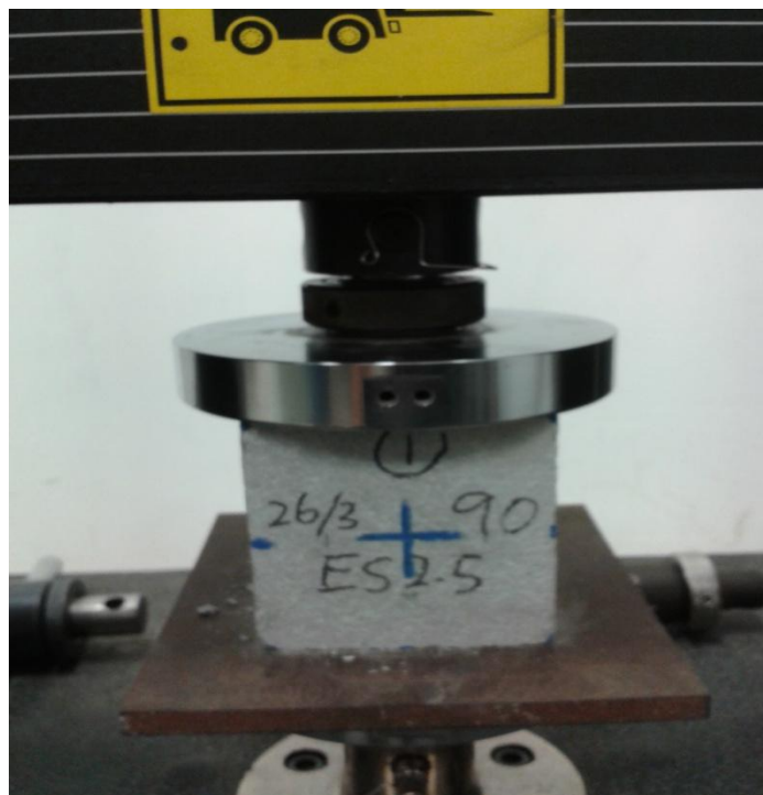
Figure 3.6: The Set Up of Apparatus for the Compressive Strength Test
