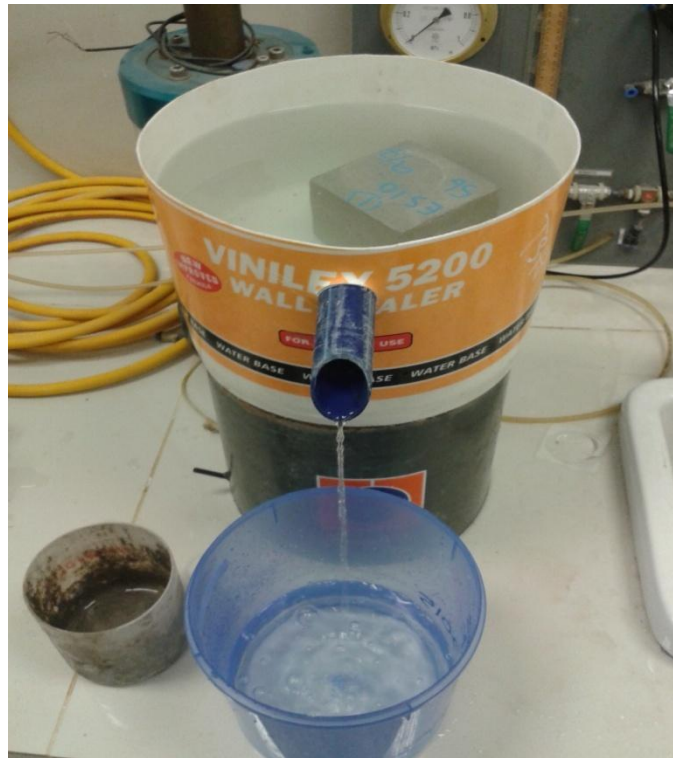
Figure 3.4: The Set Up of Apparatus for Porosity and Water Absorption Test as prescribed in BS 1881-122
