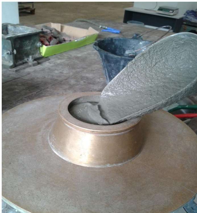
Figure 3.1: Set up of Flow Table Spread Test
