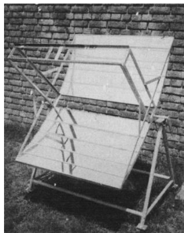
Figure 2.11: Experimental solar concentrator consisting of a series of flat panels of different sizes. (Singh and Liburdy, 1993).
