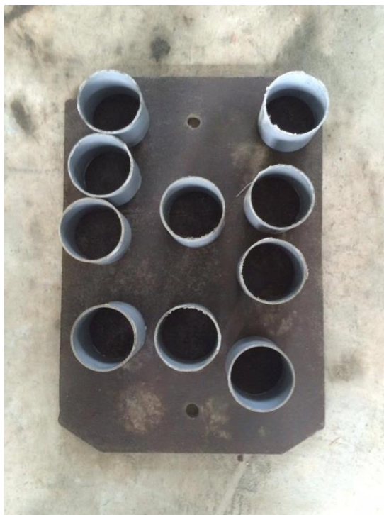
Figure 3.14 Mortar Cylinder Moulds
