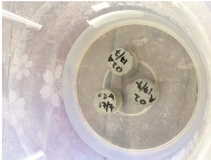
Figure 3.21 Water Absorption Test
