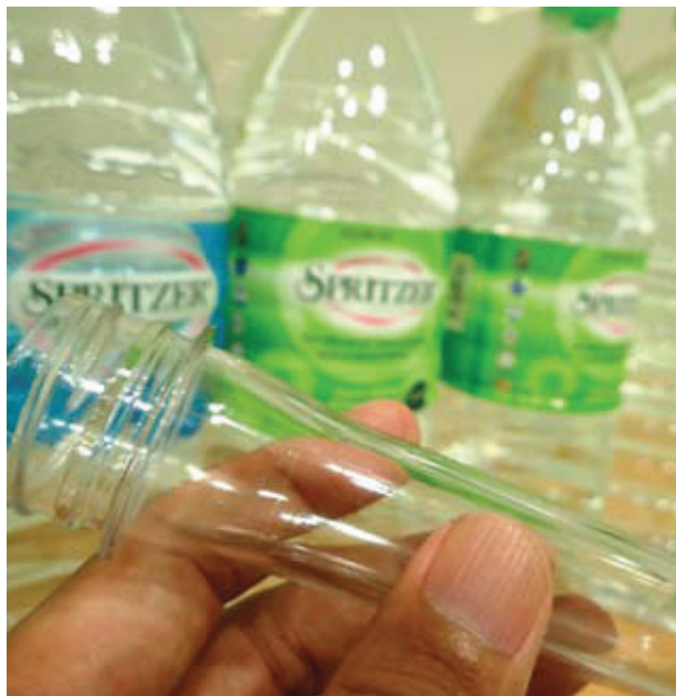
Figure 4. A PET preform looks similar to laboratory test tubes but it has preformed threads. It is placed into a blow moulding machine and the tube part is "blown" to the shape a bottle. The process produces PET bottles that are thin, light-weight and durable. Fully formed PET bottles are shown in the background.
