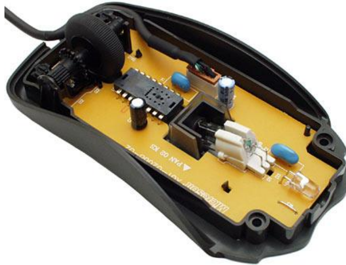
Figure 1.2 Optical Mouse, with top cover removed
