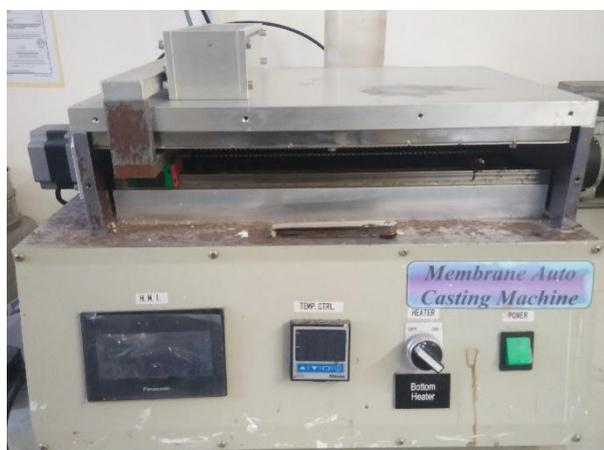
**Figure B12: Membrane Auto Casting Machine**
