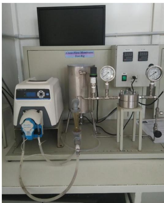
**Figure B6: Cross Flow Filtration Test Rig**
