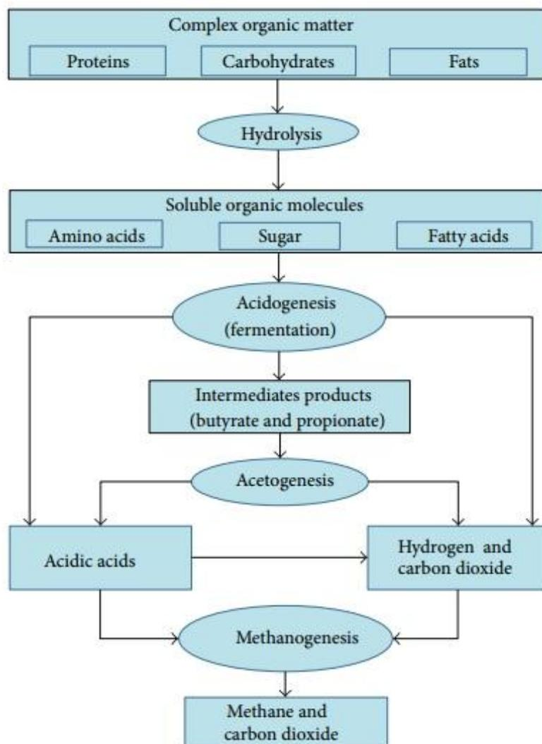
**Figure 2.5 Different Stages at Anaerobic Digestion Processes (Abdelgadir et al., 2014)**
