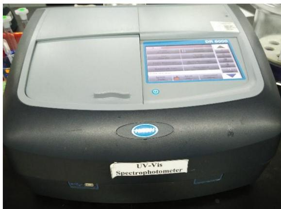
**Figure B4: UV-Vis Spectrophotometer (DR 6000)**
