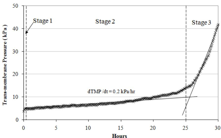
**Figure 2.3 TMP Rising Pattern during Membrane Fouling Occurrence (Yoon, 2016)**
