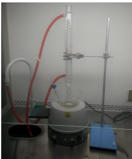
**Figure A2: Dope Preparation Set-up**
