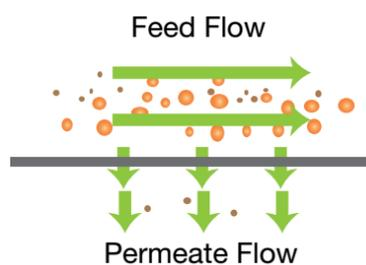
**Figure 2.1 Cross Flow Filtration Mode (Wang and Zhou, 2013)**
