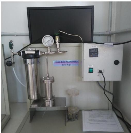
**Figure B7: Dead End Filtration Test Rig**
