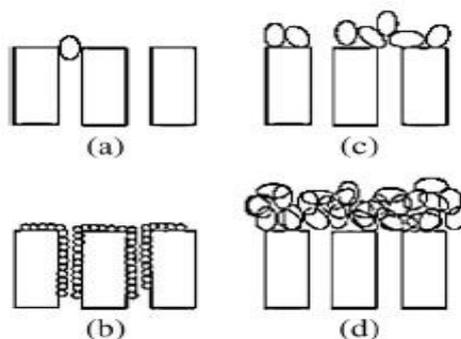
**Figure 2.4 Diagram of (a) Complete Blocking (b) Standard Blocking (c) Intermediate Blocking (d) Cake Filtration (Mutanim et al., 2012)**
