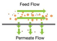
Figure 2.1 Cross Flow Filtration Mode (Wang and Zhou, 2013)
