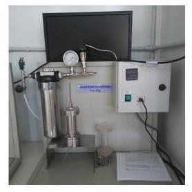
Figure B7: Dead End Filtration Test Rig
