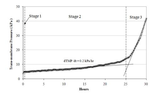
Figure 2.3 TMP Rising Pattern during Membrane Fouling Occurrence (Yoon, 2016)
