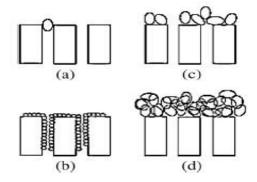
Figure 2.4 Diagram of (a) Complete Blocking (b) Standard Blocking (c) Intermediate Blocking (d) Cake Filtration (Mutanim et al., 2012)
