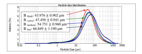
Figure 4.1 Microbial Floc Sizes Distribution of Different Anaerobic Hybrid Bioreactors in Terms of Volume
