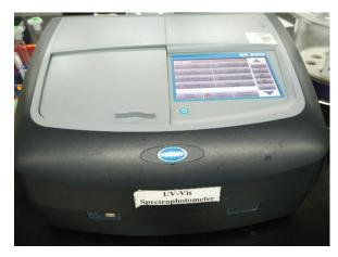
Figure B4: UV-Vis Spectrophotometer (DR 6000)
