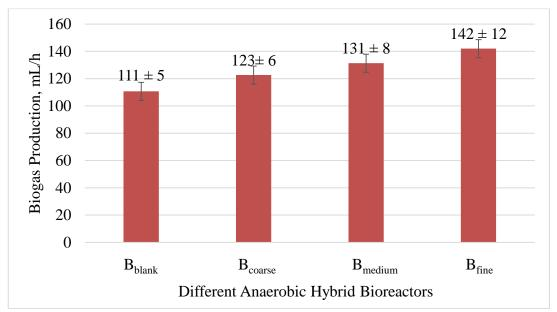
Figure 4.4 Biogas Production in Various Anaerobic Hybrid Bioreactors Added With Different Sizes of PAC
