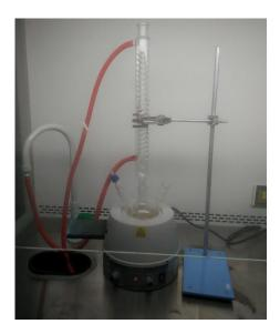
Figure A2: Dope Preparation Set-up
