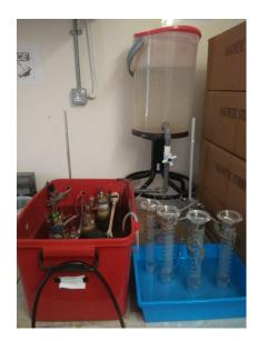
Figure A1: Four 1 L Anaerobic Bioreactors Connected with Biogas Collectors & Water Tank
