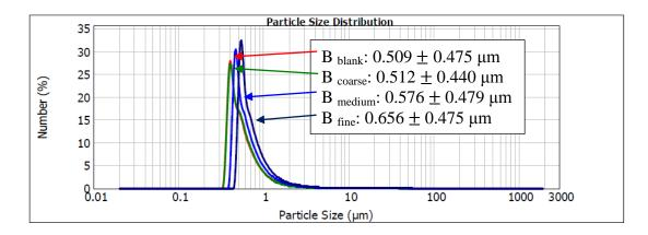
Figure 4.2 Microbial Floc Sizes Distribution of Different Anaerobic Hybrid Bioreactors in Terms of Number
