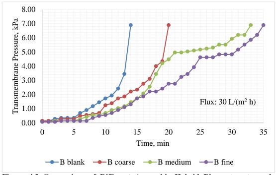
Figure 4.3 Comparison of Different Anaerobic Hybrid Bioreactors towards Membrane Fouling Control
