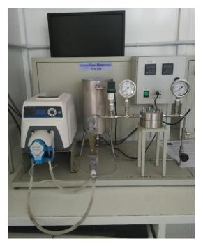
Figure B6: Cross Flow Filtration Test Rig
