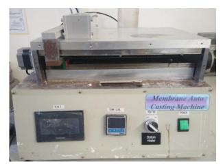
Figure B12: Membrane Auto Casting Machine
