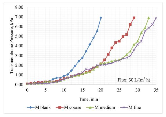
Figure 4.5 Comparison of Various PES Hybrid Membrane Incorporated with Different Sizes of PAC towards Membrane Fouling Control
