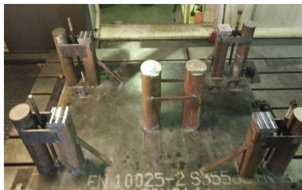
Figure 4.38: Real view of redesigned jig and fixture
