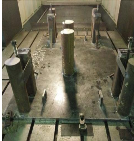
Figure 4.39: Redesigned jig clamping onto the machine table
