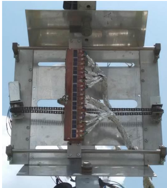
Figure 6.9: Experimental setup of the high solar flux scanner to measure solar flux distribution of NIDC prototype consisting of 96 flat facet mirrors with a dimension of 20 cm × 20 cm each and focal distance of 210 cm.
