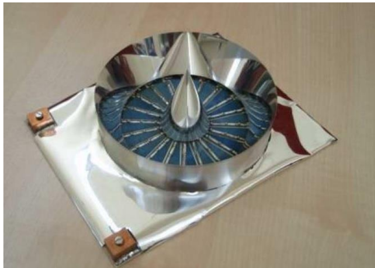
Figure 2.7: Radial large area Si-cell receiver with secondary optics (Vivar et al., 2009).
