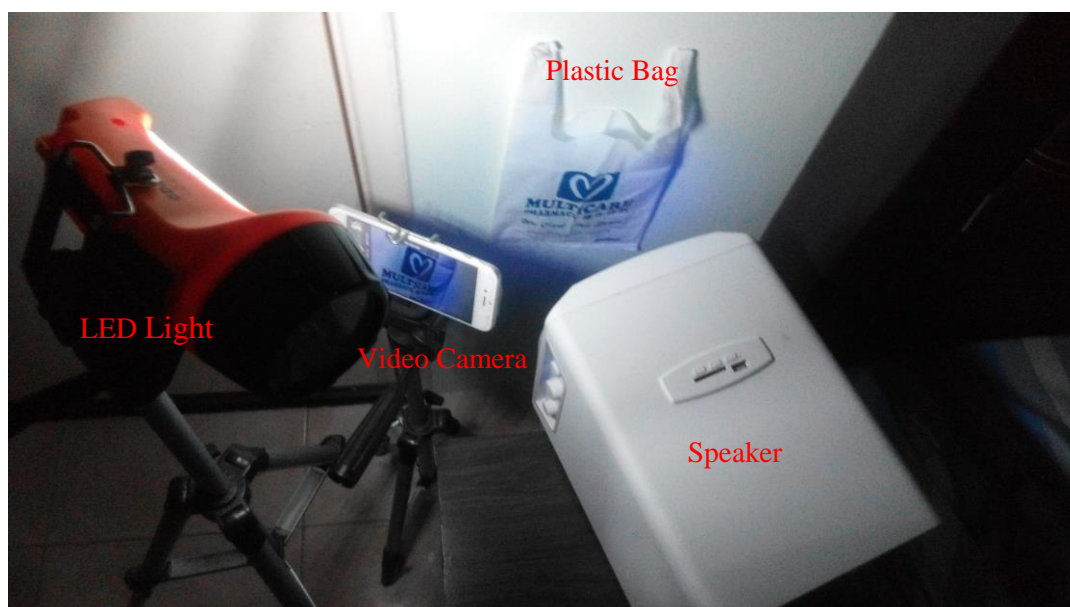
Figure 3.11: Plastic Bag(V,MM) Experiment Setup
