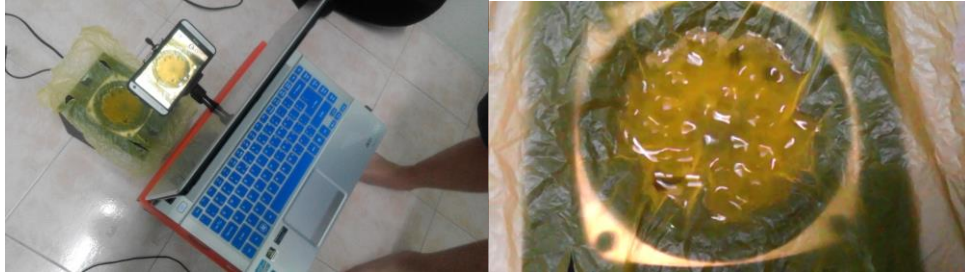
Figure 4.1: Water Ripple Experiment Setup
