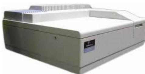
Figure 3.5: Perkin Elmer Lambda 35 UV-Visible Spectrophotometer
