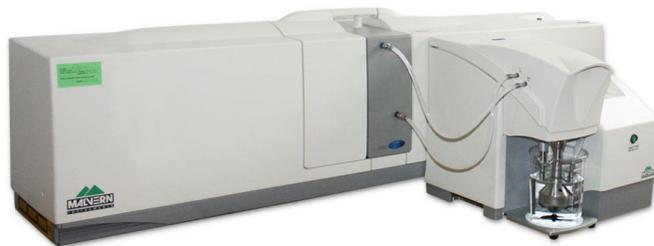
Figure 3.7: Malvern Particle Size Mastersizer 2000
