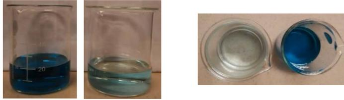
Figure 4.15: Malachite green dye solution before and after degradation.
