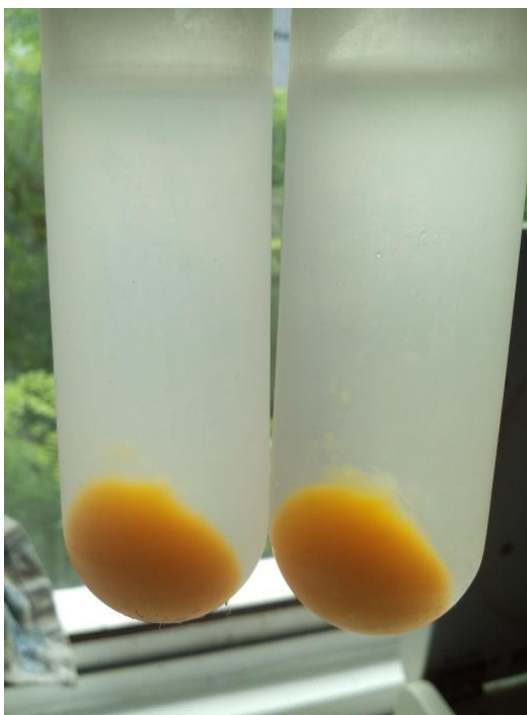
Figure 3.2: The resulting protein pellet after centrifugation of pumpkin crude extract after ammonium sulphate precipitation.
