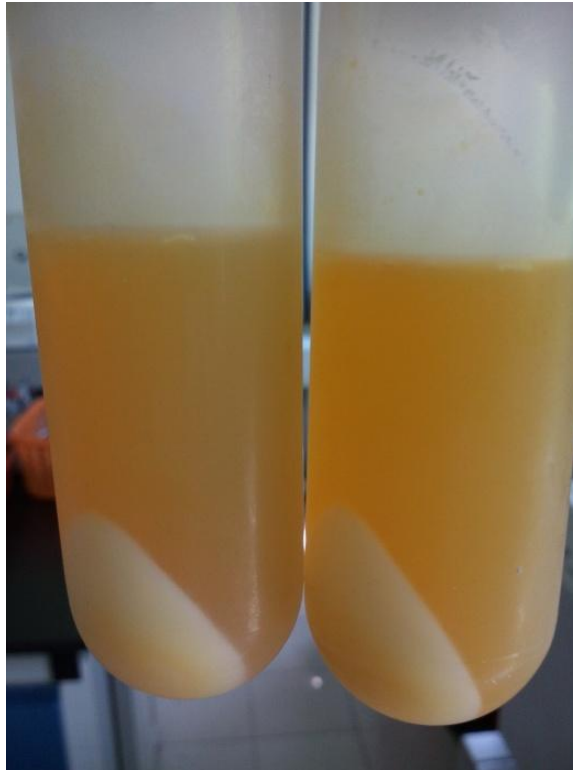
Figure 3.1: The resulting solutions after centrifugation of the blended and filtrated pumpkin crude extract.
