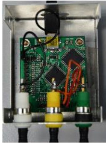
Figure 3.3: The data acquisition module. The green colored connector serves as the input of the signal channel, the yellow colored connector serves as the input of the reference channel and the white colored connector serves as the input of the ground channel.
