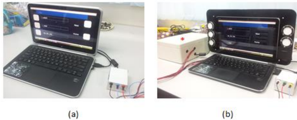
Figure 3.4: BCI systems with two different stimulators. The small unit on the right of both pictures is the EEG acquisition module. (a) BCI systems with LCD stimulator. (b) BCI systems with LED stimulator. An extra piece of hardware (denoted by *) was required to control the flashing frequency of the led flicker.
