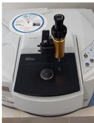
F2: Nicolet iS 10 ATR FTIR spectrometer
