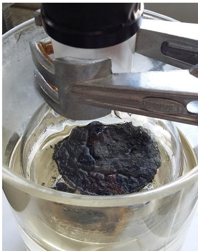
Figure 3.5: Floating coagulated RGO after 24 hours hydrazine reduction
