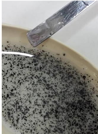
Figure 3.8: 3% weight oven dried RGO /DGEBA mixture hand stirred for 30 minutes
