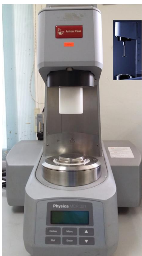
Figure 3.13: Anton Parr MCR301 rheometer (inset: side view of inserted 25 mm parallel plate spindle at a fully raised position)
