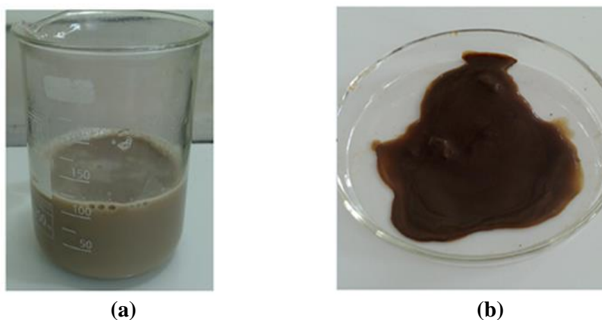
Figure 3.2: Mixture a) turns milky yellow-brown colour after addition of \text{H}_2\text{O}_2 , b) turns into a dark brown coloured GO gel after HCL wash
