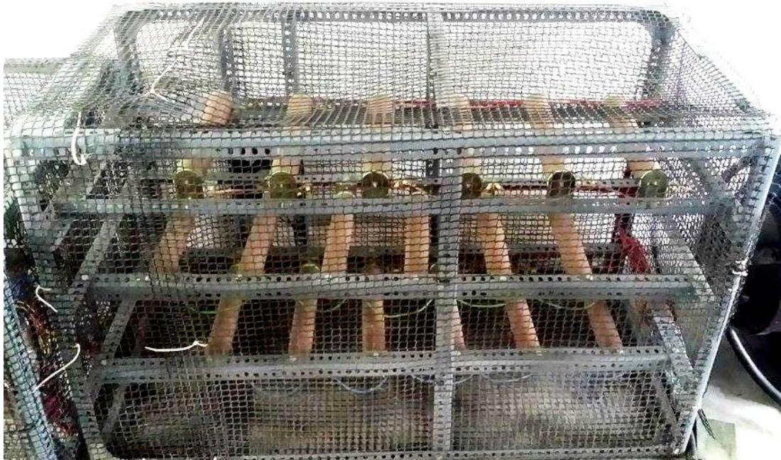
Figure 3.14: Load bank used in the experimental
