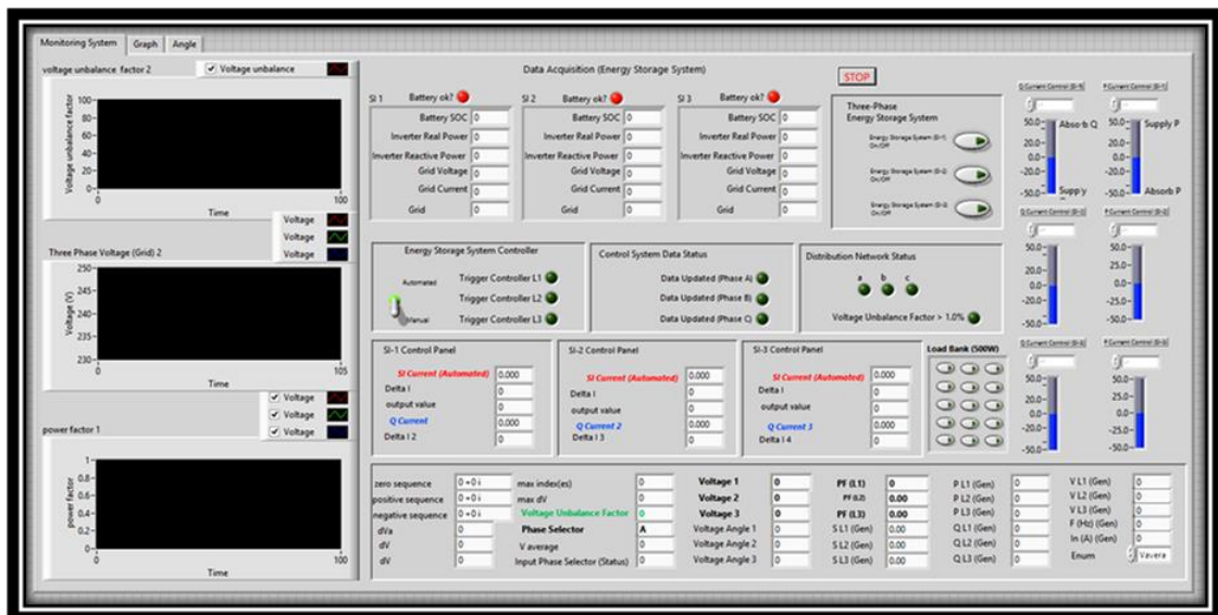
Figure 4.8: Graphical User Interface of the Energy Storage System
