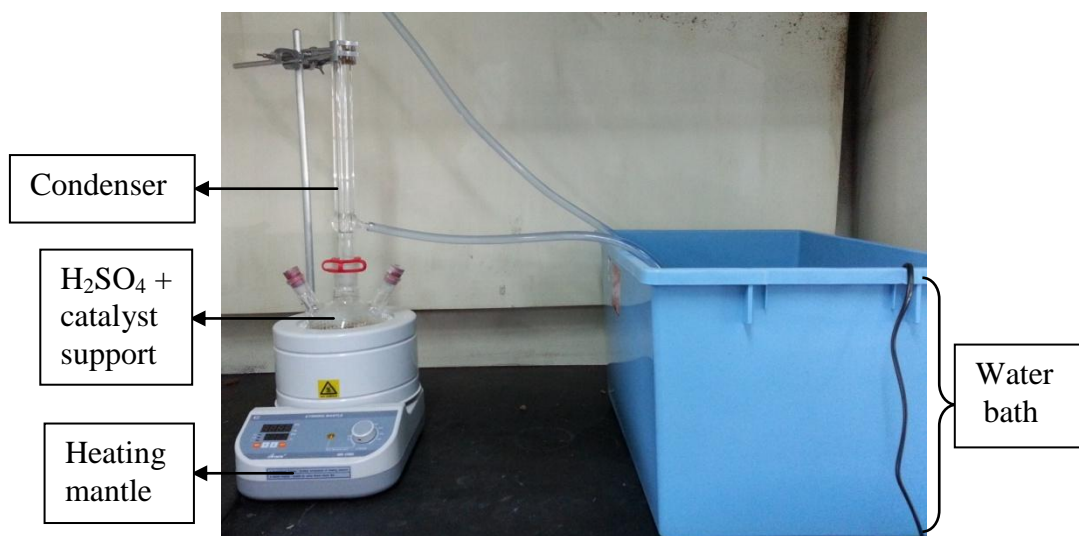
Figure 3.1: Apparatus setup for catalyst sulfonation.
