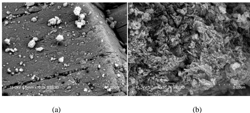
Figure 4.1: SEM micrographs of (a) original \text{Al}_2\text{O}_3 and (b) sulfonated \text{Al}_2\text{O}_3 .
