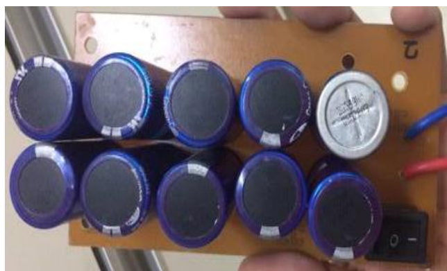
Figure 3.10: The supercapacitor in parallel module
