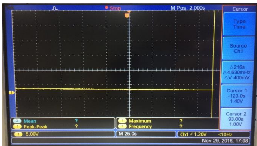
Figure 4.20: Discharging process of case 9 (with supercapacitor)
