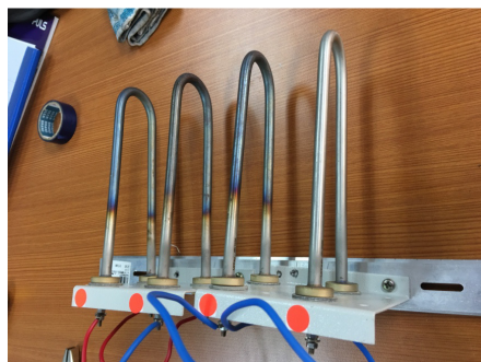
Figure 4.13: Heater is used to simulate the load
