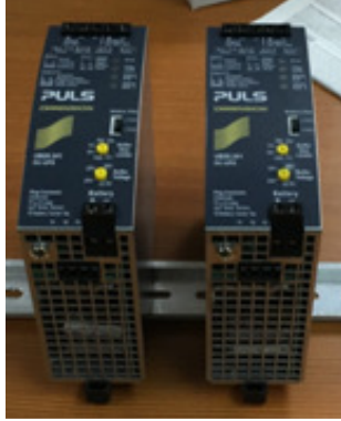
Figure 4.5: Intelligent Power Controller
