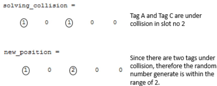
Figure 4.2.3: Example of Solving Collision by Generate New Random Number in Dynamic Based
