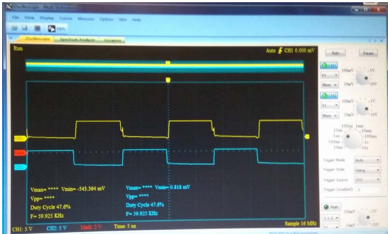
Figure 5.2: The oscilloscope showing two pulse wave as verification
