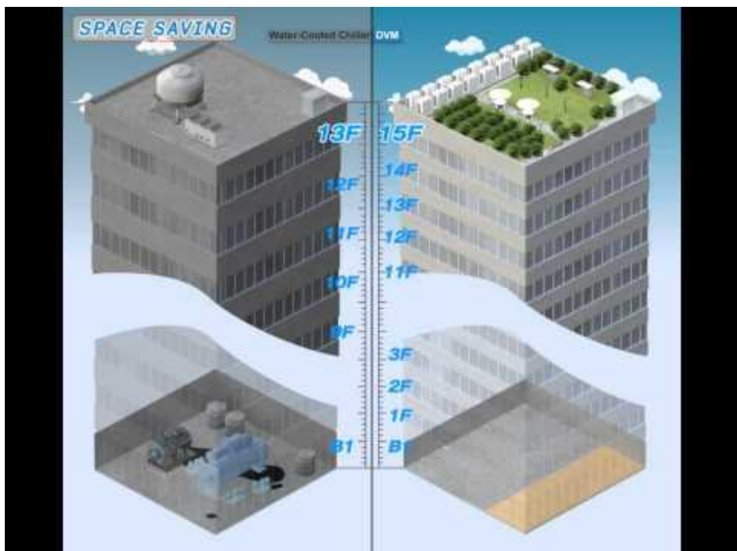
Figure 2.11 Plant room comparison between chilled water plant and VRF system
