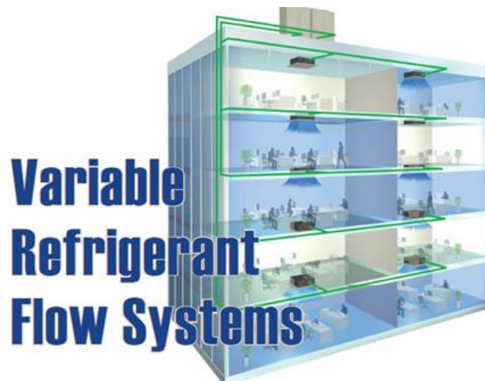
Figure 2.9 Schematic diagram of VRF system
