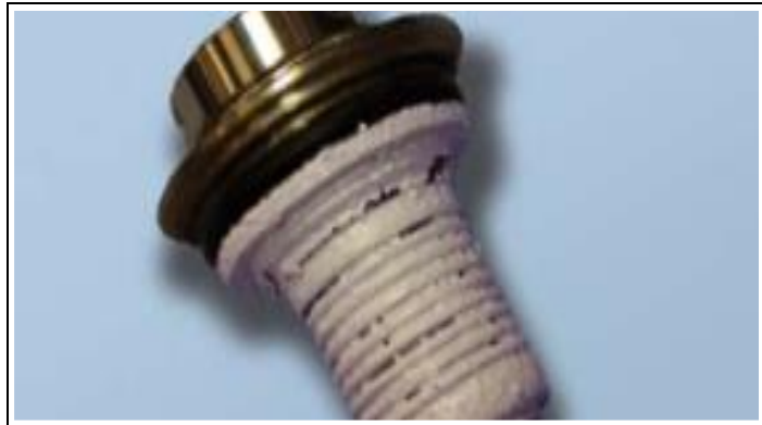
Figure 41: Mechanical Seal Spring with Solidify Fats
