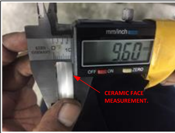
Figure 42: Ceramic Seal Thickness Reading with a Caliper.
