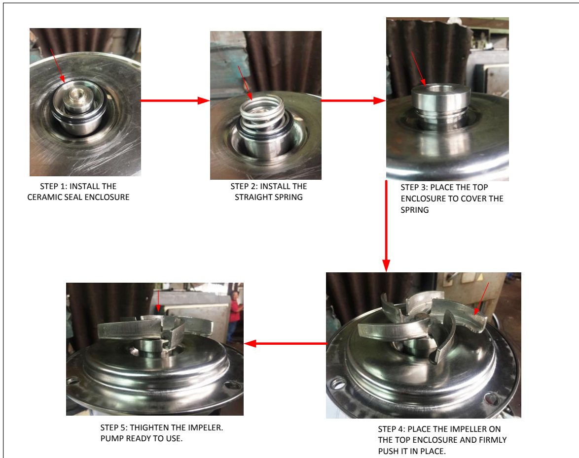
Figure 39: Steps in installing Mechanical Seal Prototype
