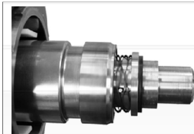
Figure 22: Installed Double Mechanical Seal (Waukesha, 2013)
