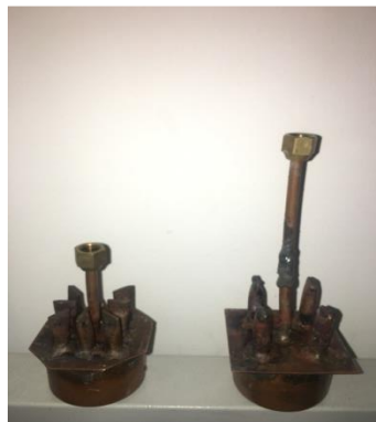
Figure 5: Vapor chamber with embedded hollow condenser tube heat sink
