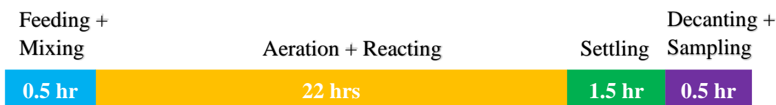
Figure 3.22: A Complete Cycle of SBR
