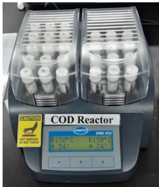
Figure 3.9: COD Heat Reactor (DRB 200, Germany)
