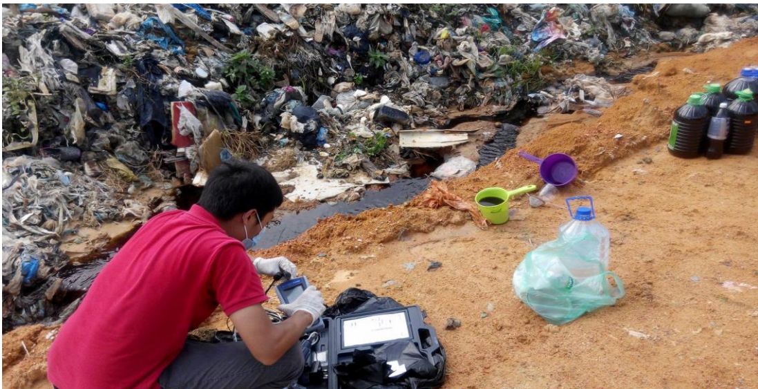
Figure 3.4: Leachate Sample On-Site Parameter Analysis Using EUTECH CyberScan PCD 650 Multi-Parameter, Singapore
