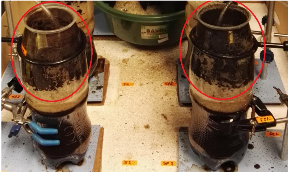
Figure 4.3: The Suspended POME Sludge and Other Solids Adhere On the Wall and The Cap of the Reactor.
