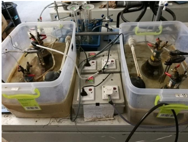
Figure A3: Hybrid Anaerobic Bioreactors operated at 55°C (left) and 35°C (right)
