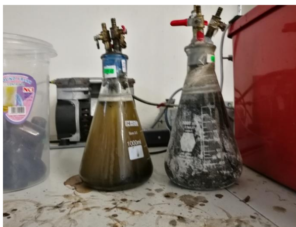
Figure A1: Hybrid Anaerobic Bioreactors operated at ambient temperature
