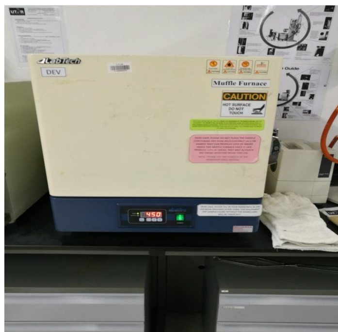
Figure B4: Muffle Furnace
