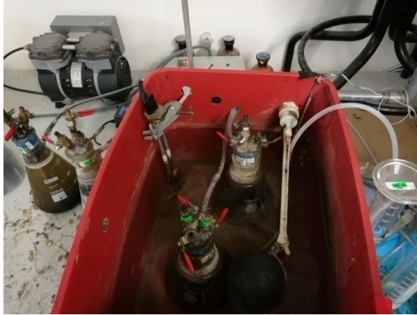
Figure A2: Hybrid Anaerobic Bioreactors operated at 45°C
