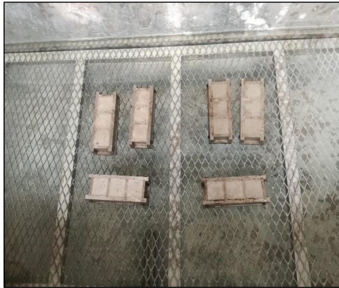
Figure 3.14 RePOFA mortar cured under hot water bath at phase one
