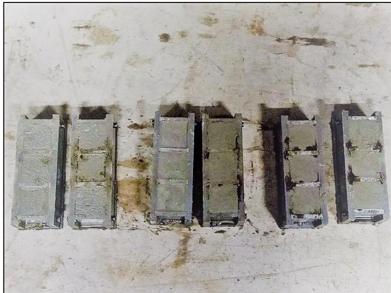
Figure 3.12 Cube moulds with fresh RePOFA mortar
