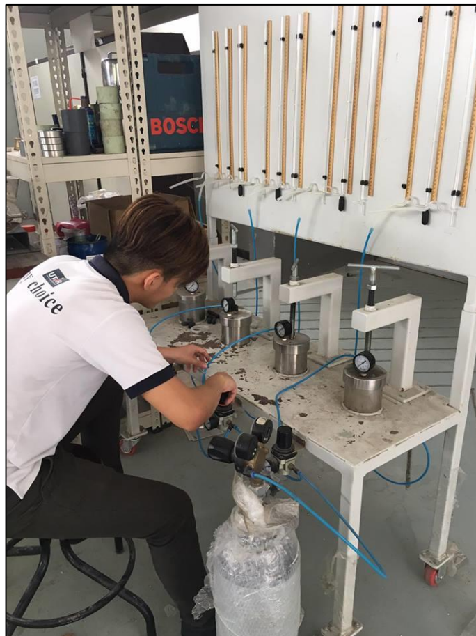
Figure 3.25 Intrinsic air permeability testing machine
