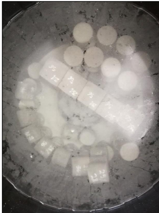
Figure 3.15 RePOFA mortar cured under ambient temperature water at phase two
