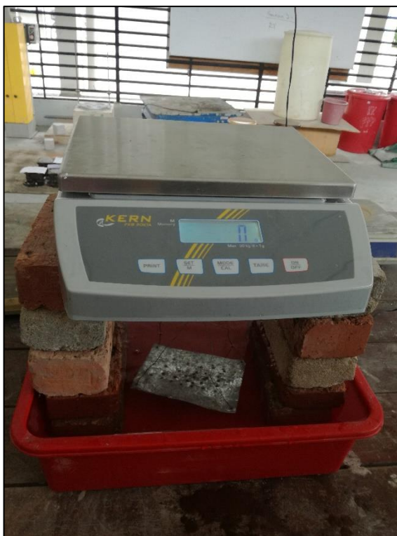
Figure 3.20 Equipment setup for density test
