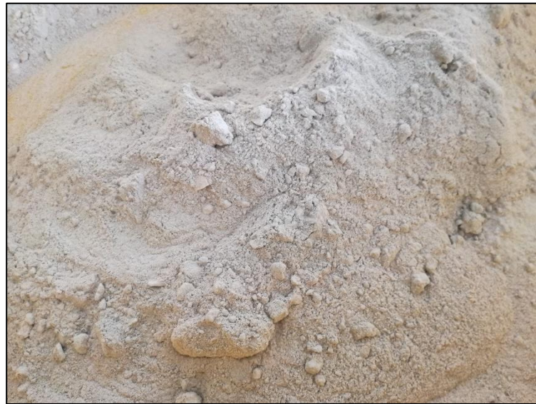
Figure 3.2 RePOFA after re-incinerating under 700°C for 3 hours
