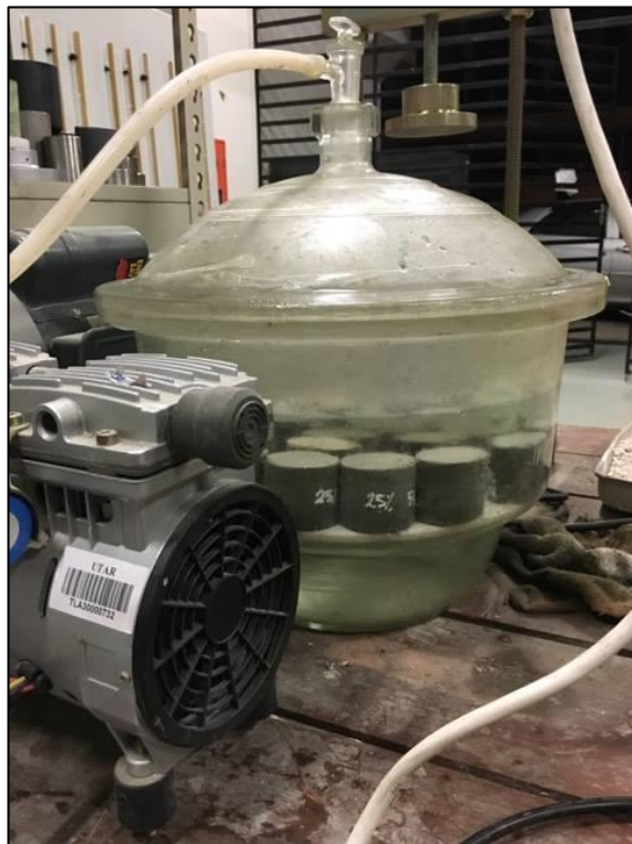
Figure 3.24 RePOFA mortars were vacuumed for 15 minutes
