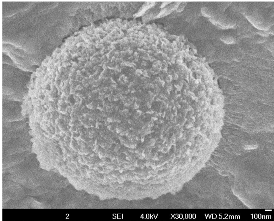
Figure 4.38: Partially-dissolved PFA particle found in G50F33P17
