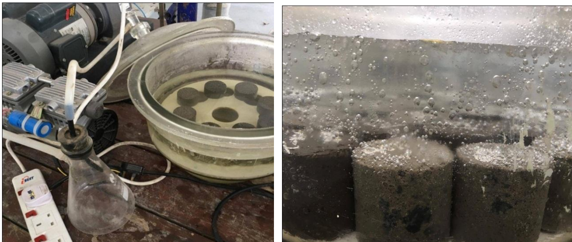
Figure 3.15: Vacuum-pressure vessel for obtaining saturated mass
