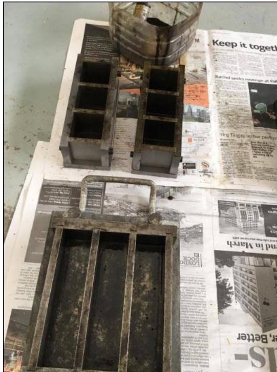
Figure 3.5: Application of demoulding oil prior to specimen casting
