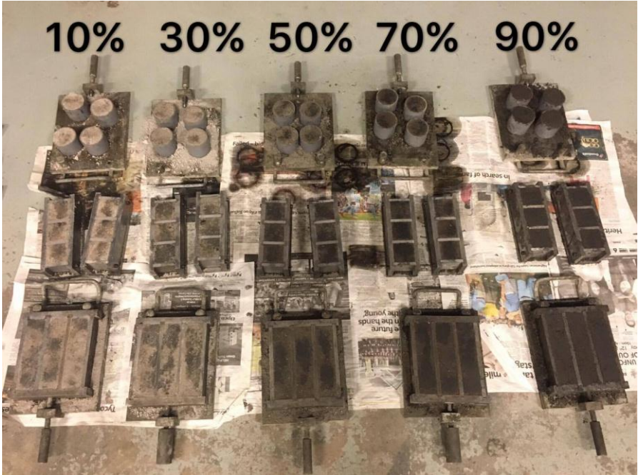
Figure 3.6: Experimental specimens with varying replacement level of GGBS
