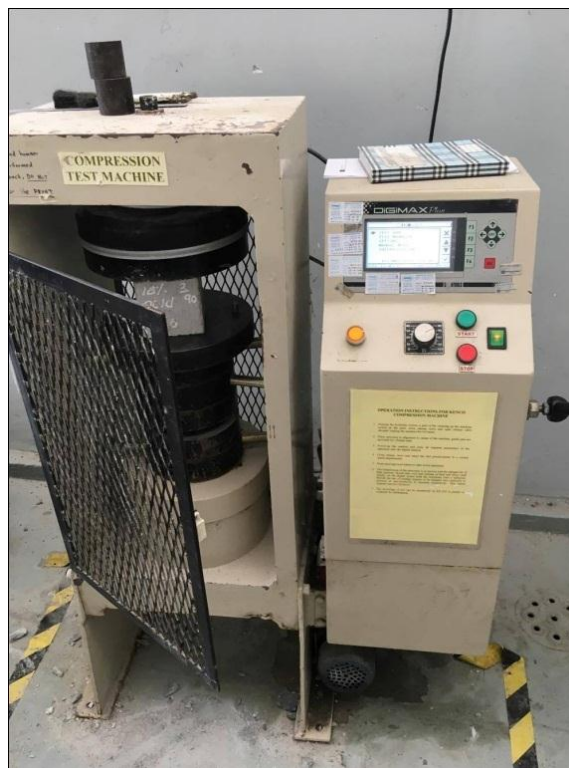
Figure 3.11: Kenco compressor testing machine
