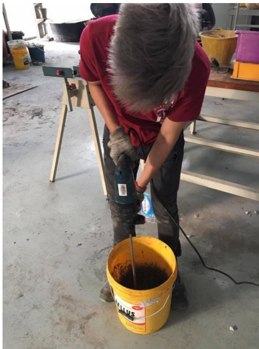
Figure 3.4: Preparation of geopolymer mortar
