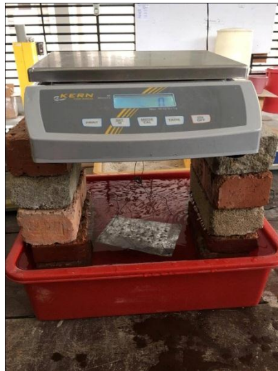
Figure 3.12: Measurement of mass in air as well as mass submersed in water
