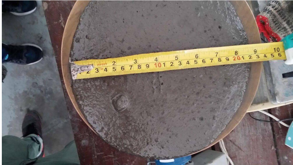
Figure 4.8: Flow table of PFA2.5:POFA0.5 with inclusion of superplasticizer
