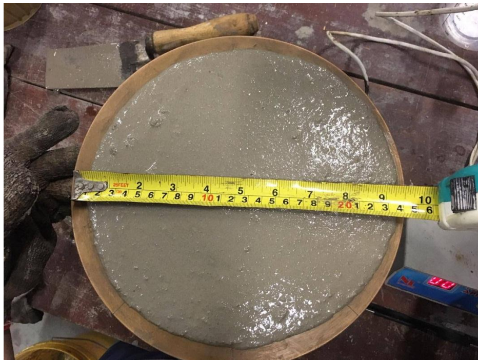
Figure 4.9: Flow table of PFA1:POFA2 with inclusion of superplasticizer
