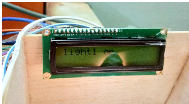
Figure 4.2.28 Status of Light On on LCD Display
