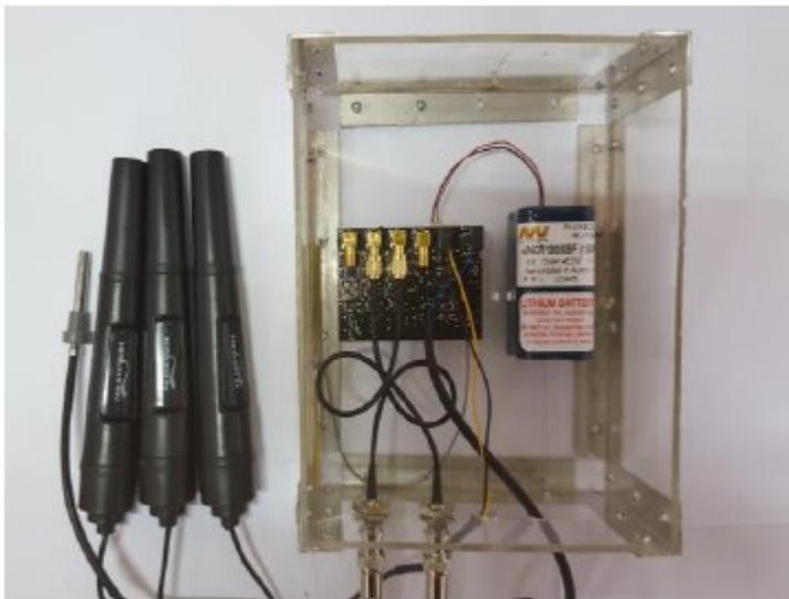
**Figure 2-1-F2: Deployment Setup with the sensors and Wasmote microcontroller board.**
