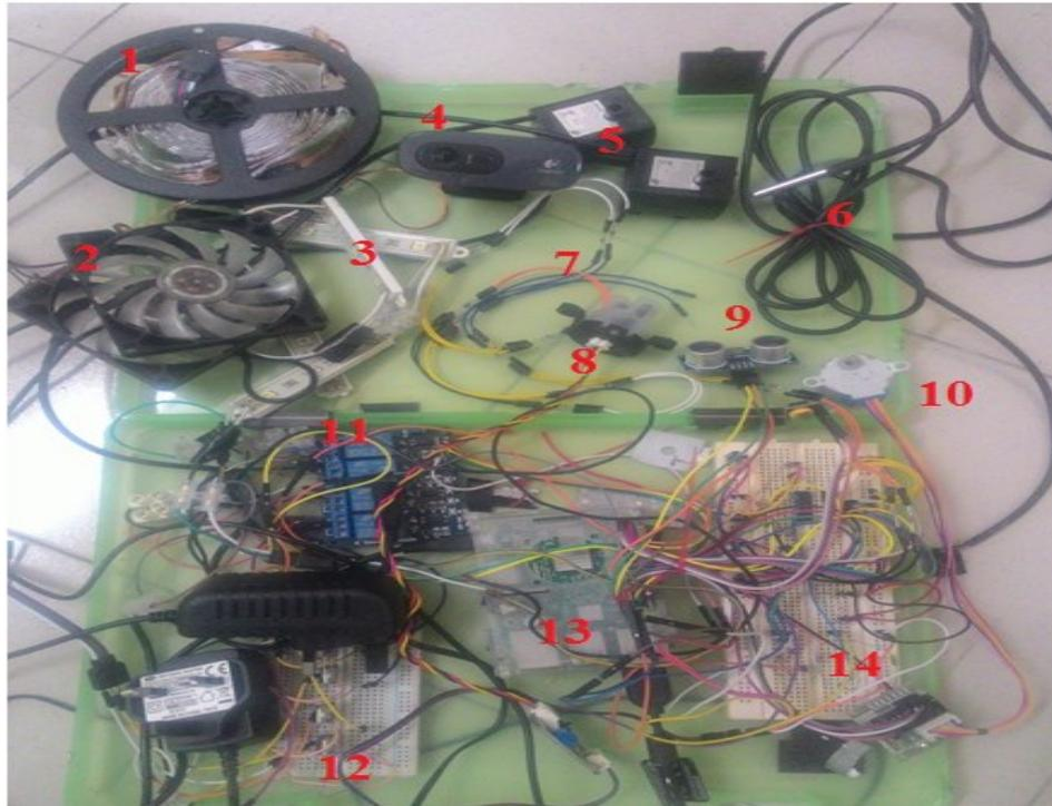
**Figure 3-1-F2: Physical connection of the components of system**
