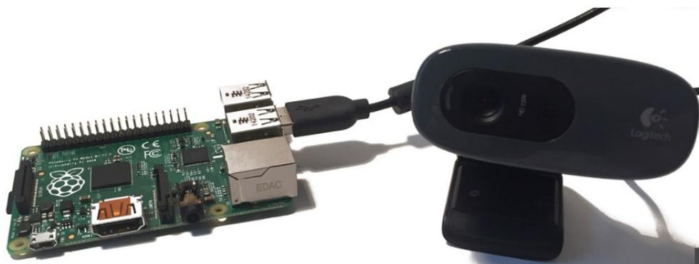
**Figure 5-0-1-F-65: Connection between C270 and Raspberry Pi**
