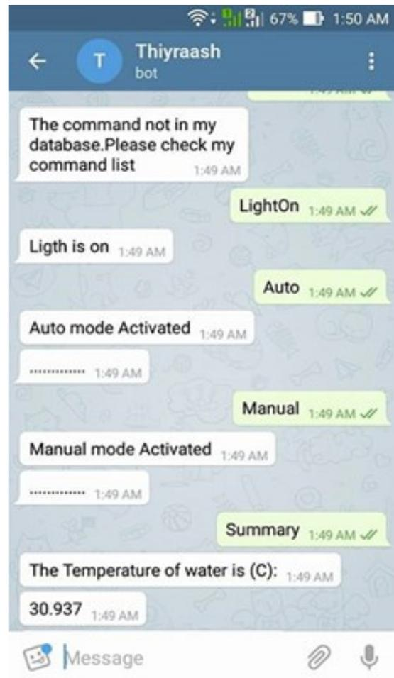
**Figure 3-1-2-F7: Example of command send from my smartphone to Pi's Telegram bot**
