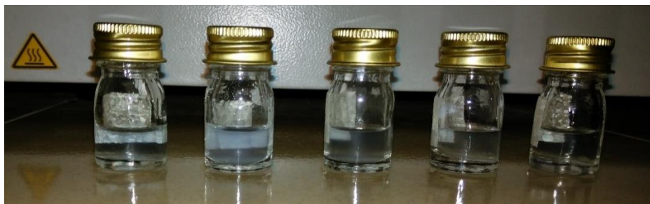
Figure 4.8: Color of different concentration of GA after incubating with \text{Na}_2\text{CO}_3 , ethanol and FC before subjecting to spectrophotometer
