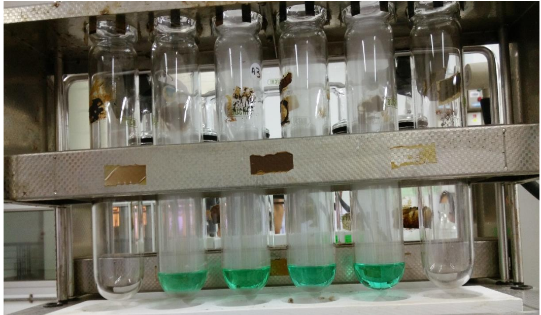
Figure 4.5: Color of the solution of control noodles and noodle samples incorporated with 5, 10 and 20 % of bell pepper in digestion tube after digestion process. (From left to right: Control, noodles with 5, 10 and 20 % of bell pepper)
