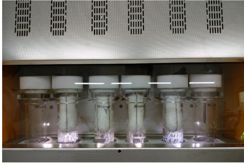
Figure 4.6: Images of fat extraction using Soxtherm analyzer
