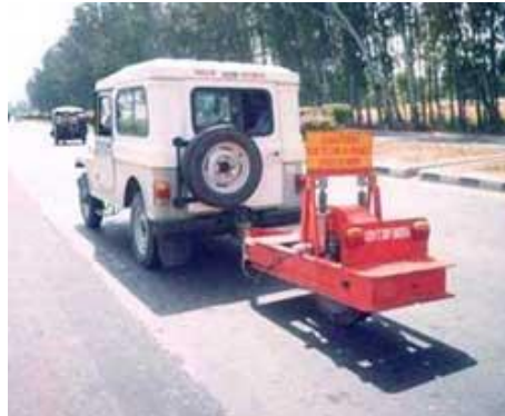
Figure 2-2 Fifth Wheel Bump Integrator
