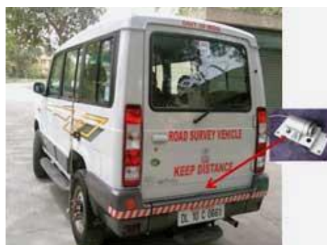
Figure 2-3 Vehicle Mounted Bump Integrator
