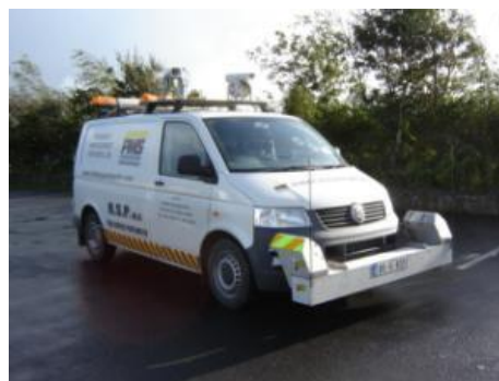
Figure 2-5 Road Surface Profiler
