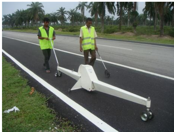
Figure 2-4 Rolling Straight Edge
