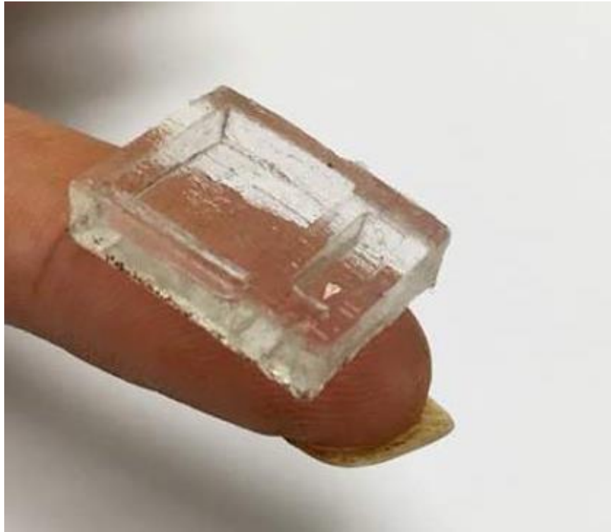
Figure 3.14: Fabricated prototype device body using IPMC
