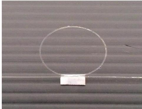
Figure 3.3: Configuration of the bend-coated fiber sensor
