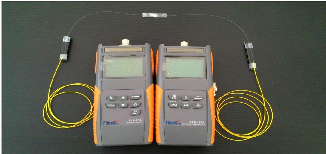
Figure 3.5: Bending loss measurement setup
