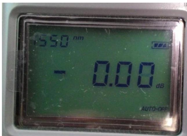
Figure 3.6: The reference value of the optical power meter is set to 0.00 dB
