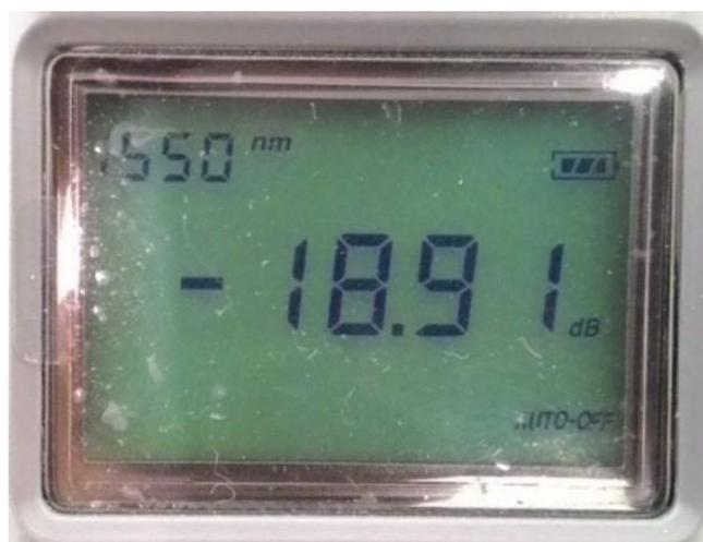
Figure 3.7: Losses display on the power meter due to the bending of fiber
