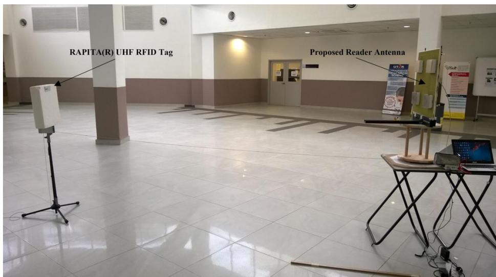
**Figure 4.4: Experimental Setup to Measure the Read Range.**
