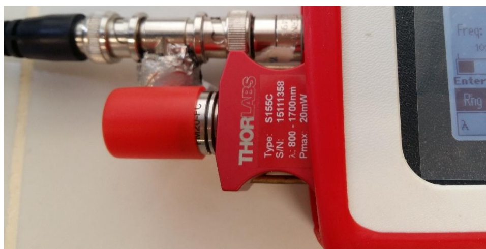
Figure 3.11: Thorlabs photodetector S155C series for measuring optical power fluctuation
