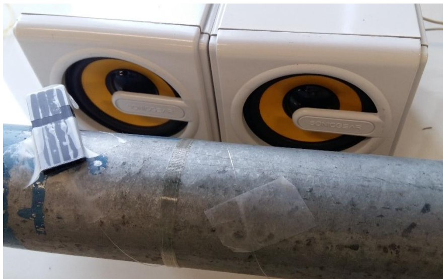
Figure 3.7: Airborne source vibration experiment setup which have a speaker control by a computer and place in front of the fibre sensor
