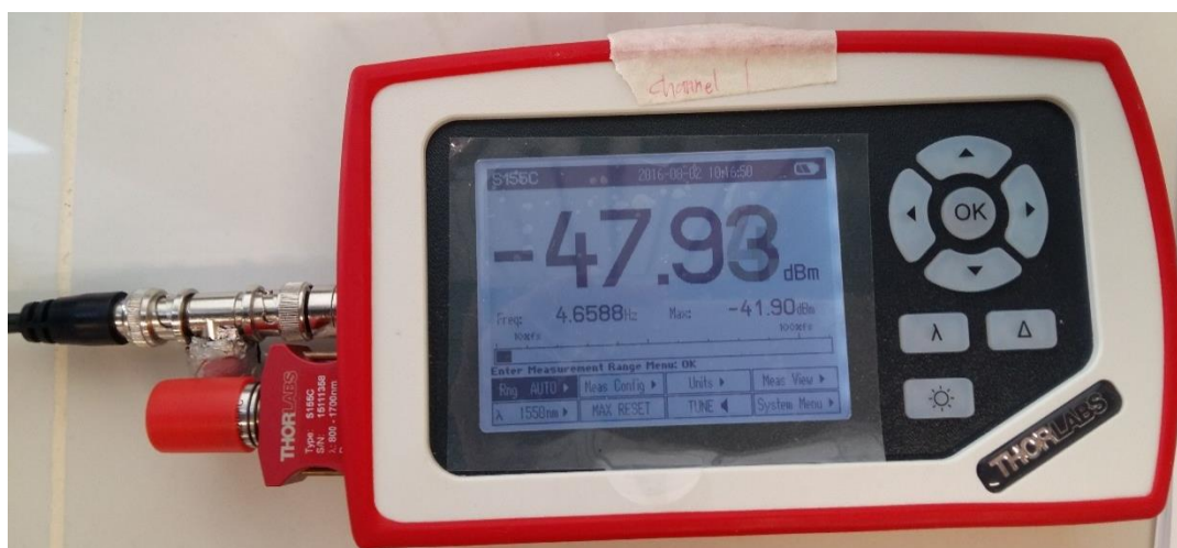
Figure 3.12: Digital optical power display meter will convert optical signal to electrical signal then transmit to digital oscilloscope to analysis
