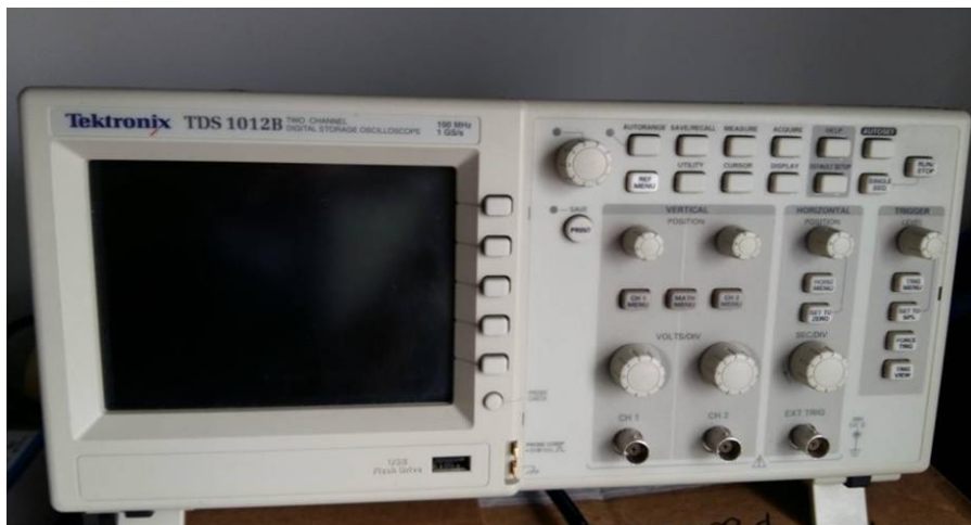
Figure 3.13: Tektronix TDS 1012B series digital oscilloscope is used as its sampling rate is 1 Gb/s which sufficient for this research
