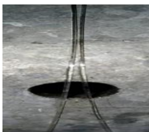
Figure 4.25 Two fibre rings on hole, but not closely touch
