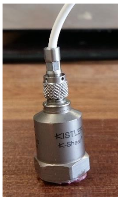
Figure 4.1: AE sensor for detecting the stress wave signal on the metal pipeline
