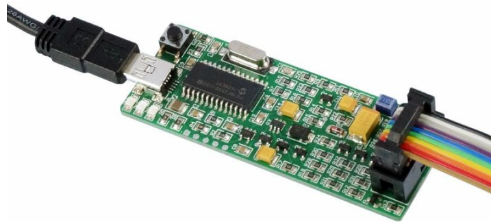
Figure 3.2: UIC00B of USB ICSP PIC Programmer
