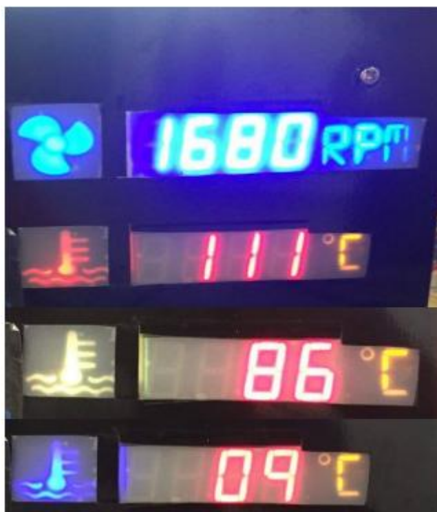
Figure 4.11: Red, Yellow and Blue Colour Indication for Different Temperature
