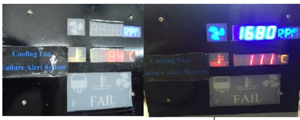
Figure 4.12: Cooling Fan On (right) and Cooling Fan Off (left)
