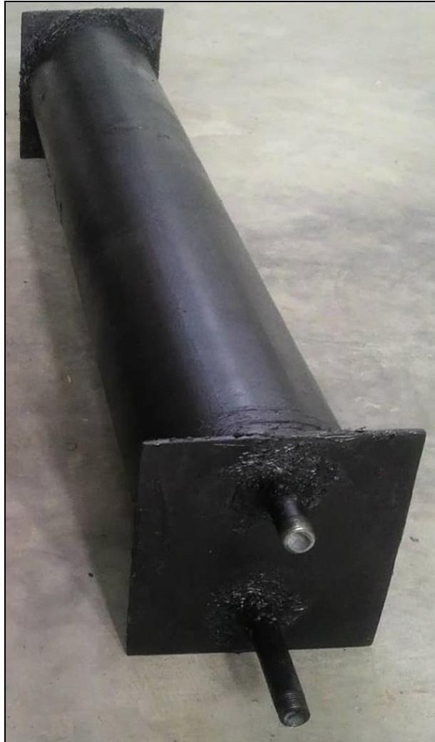
Figure 3.21: Water Tank with Piping System
