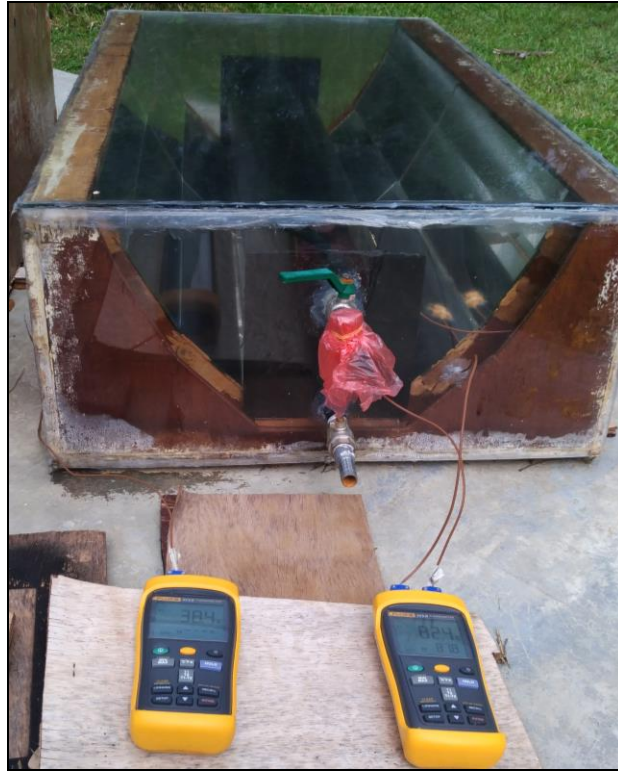
Figure 3.23: Tank surface, Water and Ambient Temperatures Data Collection
