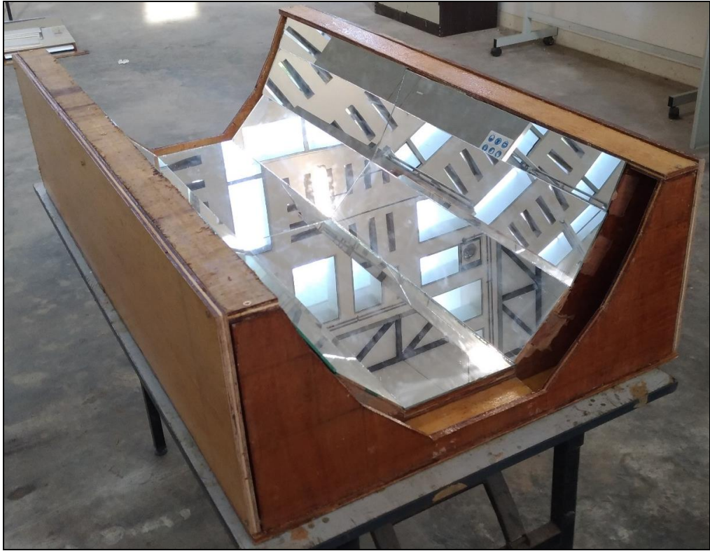
Figure 3.20: Mirrors were attached to the Supportive Frame
