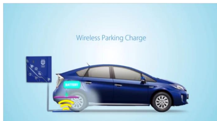
Figure 2.1 Graphic of a wireless parking charge setup built into a parking space. Image courtesy of Toyota. (Corporation., 2018)
