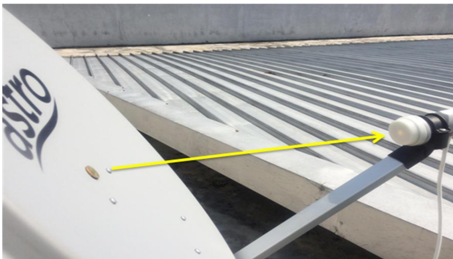
Figure 3.8 Reflection of the sun off the shiny coin onto the antenna feed.
